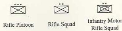
Figure 3. A sample of the types of icons used to convey structural information about the dynamic objects displayed on the Map. For the military intelligence application, the dots indicate the size of the object (platoon or squad in this case), and the contents of the rectangle indicate the type of the object (rifle or infantry motor rifle).
